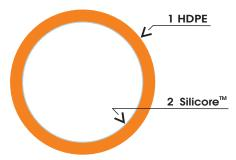
Wall thickness and material classify the duct as a Direct Burial (DB). Installation methods and conditions are described in the Installation manual.
